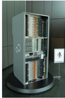
An array of the quadrillion computer "K computer" in the computer room (left). One chassis is equipped with 24 system boards (right).
